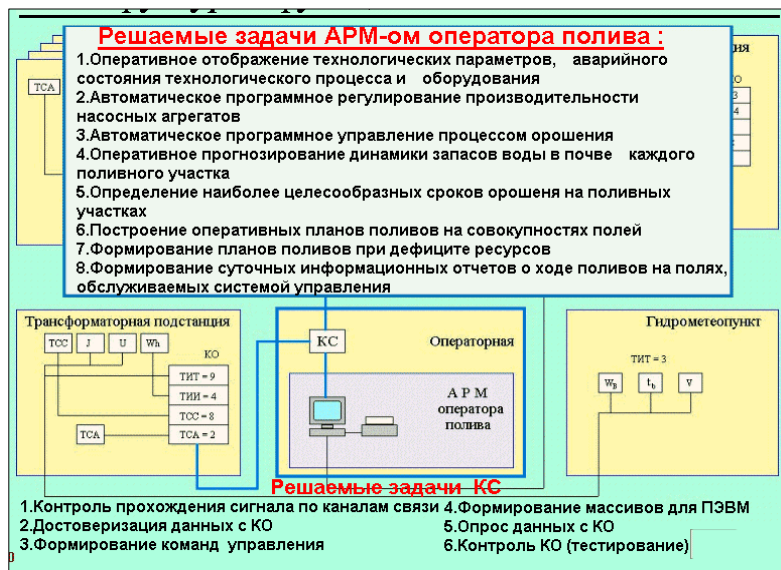
Fig 2: Structural and functional diagram of the automated process control system for irrigation.
